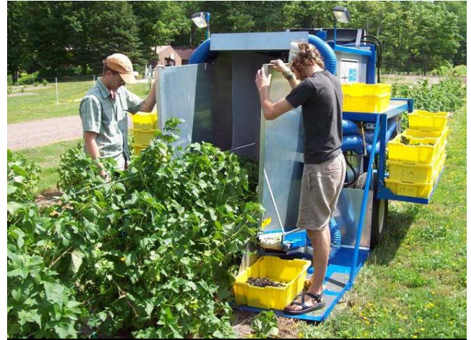
Photo 1. Mechanical harvest of black currants is possible with a blueberry harvester shown here. On-going research is helping develop currants as a viable crop for Bayfield growers.
